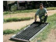
▲ With a little black paint, the solar panel is finished.
