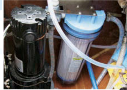
▲ Eruç used a machine to make salty ocean water safe to drink.
